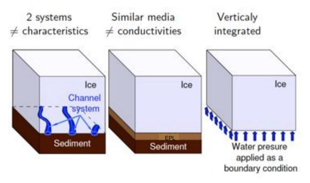
Based on Darcy equation for both in the Inefficient Drainage System (IDS) and the Equivalent Porous Layer (EPL)
