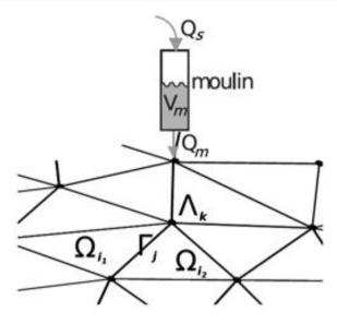
Based on the empirical Darcy-Weisbach law (turbulent flow) for both the water sheet and the channels. Channels stands on the edge of the surface elements.
