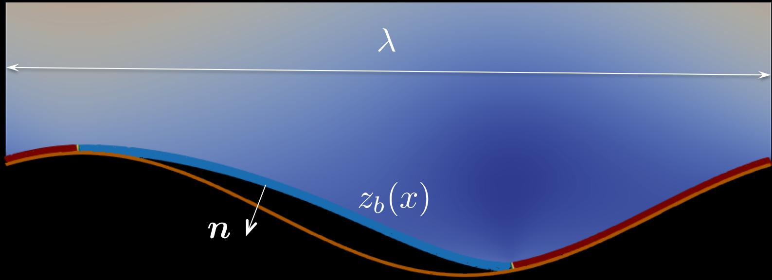
$$\left. \begin{aligned} \tau_b &= \frac{1}{\lambda} \int_0^\lambda \sigma_{nn} n_x ds = \frac{1}{\lambda} \int_0^\lambda \sigma_{nn} \frac{\partial z_b}{\partial x} dx \\ u_b &= \frac{1}{\lambda} \int_0^\lambda u dx \end{aligned} \right\} \rightarrow \tau_b = f(u_b, N) \quad N = p_i - \bar{p}_w$$
